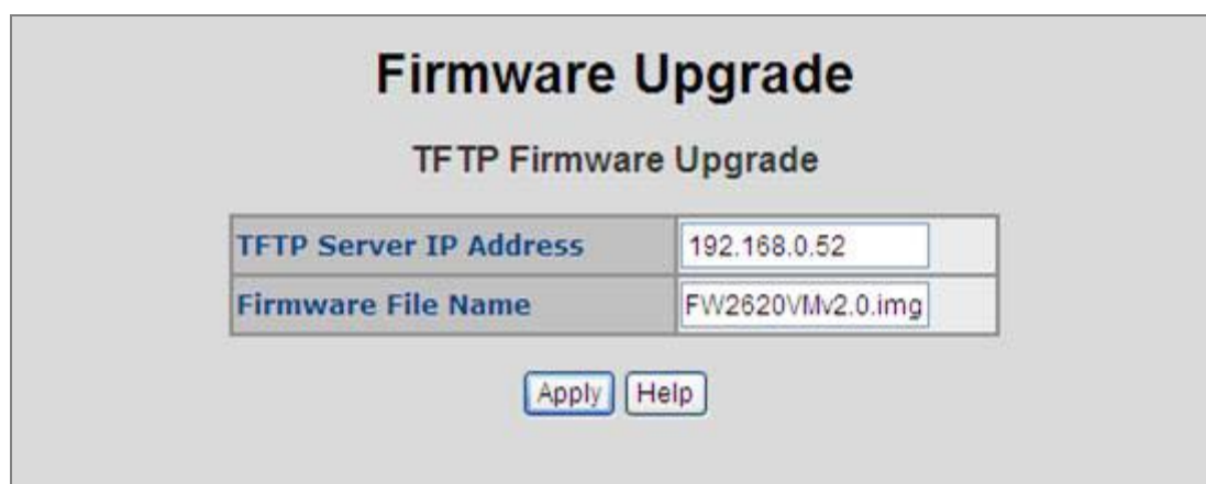
Figure 4-2-9: Firmware Upgrade interface
